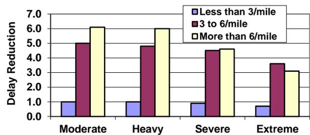
The effect of the signal coordination projects was to reduce delay by 21.7 million person hours, approximately one percent of the street delay (Exhibit B-21). This value is combined in the operational effects summary at the end of this section.
