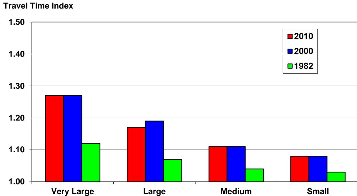
Note: The Travel Time Index is a ratio of average peak period to free-flow travel time. A value of 1.30 indicates a free-flow trip of 20 minutes takes 26 minutes in the peak due to heavy traffic demand and incidents.
